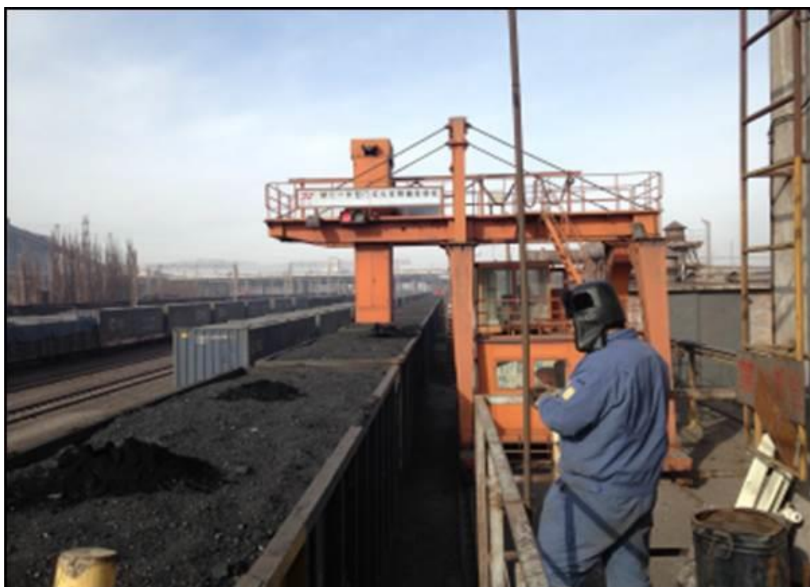
Auto sampler from the railway wagons.
