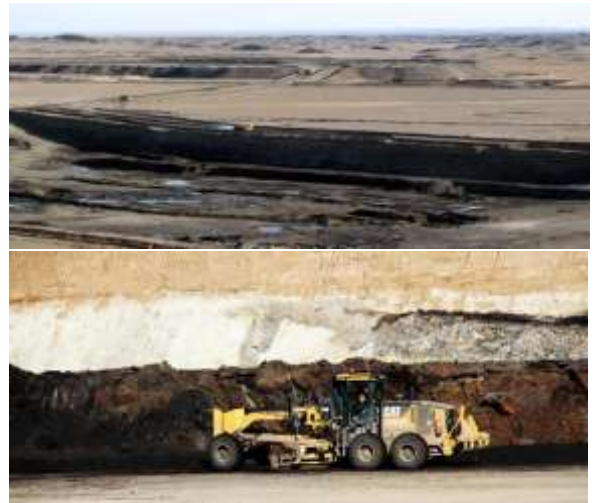
Figure 3 and 4: Top – Panoramic view of the box cut at the BNU Mine. Bottom: Digger working exposed coal seam at base of box cut. Source: Guildford
